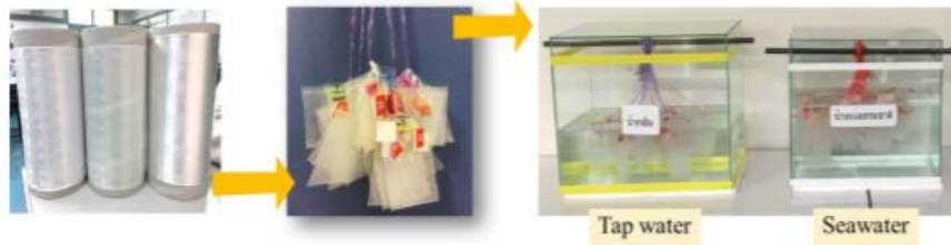
Figure 3 Degradability of POM/PLA fibers in sea water and tap water
