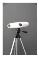
Figure 8.2 Stereo camera Axios Cambar B2, Axios 3D, Oldenburg, Germany.
