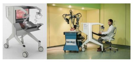
Figure 16.20 Robin STIFF-FLOP console: CAD model and integration with Robin Heart [16].
