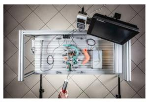
**Figure 17.4** Illustration of the potential use of the phantom environment for capturing and analyzing the action of the robotic arm. Experiments can use the STIFF-FLOP arm directly inside such a system.
