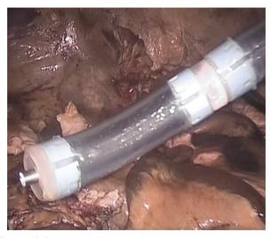
Figure 19.4 Flexible STIFF FLOP camera during cadaver tests.
