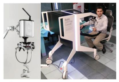
**Figure 16.7** Haptic *RobinHand L* – mobile version and the version adapter for the STIFF-FLOP console.
