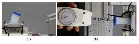
**Figure 3.14** (a,b) Test setup for measuring the individual-chamber braiding influence on module bending elongation by external force, respectively.
