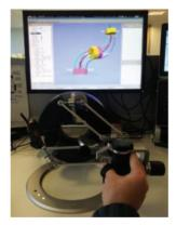
**Figure 9.1** Example of a haptic device used to receive the motion request for the robotic tool (Omega 7 from Force Dimension<sup>1</sup>). For description refer to Chapter 16.
