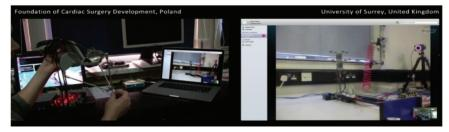
**Figure 16.13** FCSD Haptic *RobinHand H* connection to the ROS system; performing telemanipulation between FCSD (at left) and UoS (at right).
