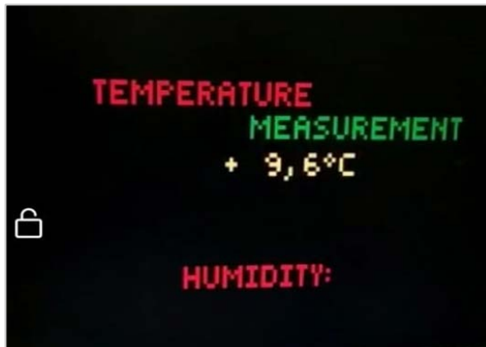
Figure 26-6 The monitored data on VGA display by interfacing with the microcontroller
