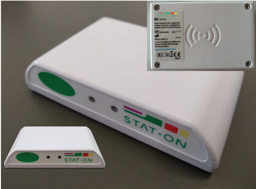
Figure 3.22 Final industrialized enclosure of the STAT-ON™ device.
