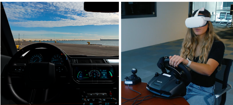
Figure 15.5 Remote cockpit implementation from first-person view (left) and third-person view (right).
