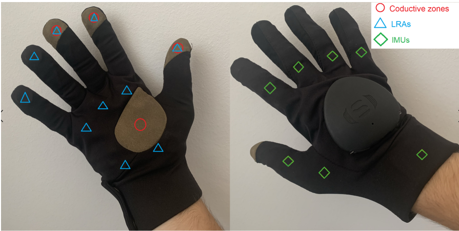
Figure 15.2 Sensors and actuators of Sensorial XR [16].
