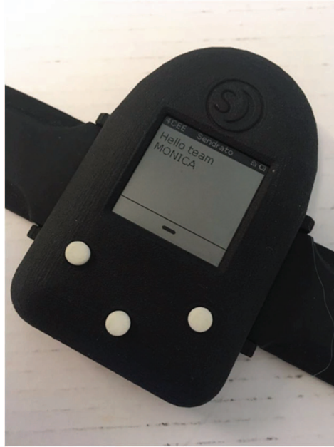
Figure 5.8 UWB-based staff wristband.
