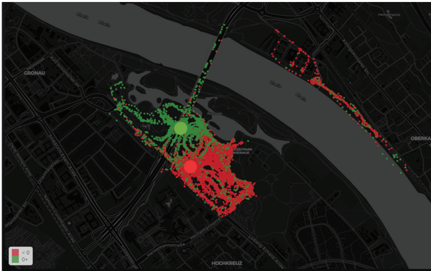
Figure 5.11 Signal coverage of two LoRa gateways (Red and Green) in the Rhein in Flammen event.
