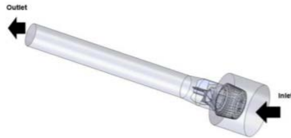
Figure 4 CAD geometry of the irrigation pump system
