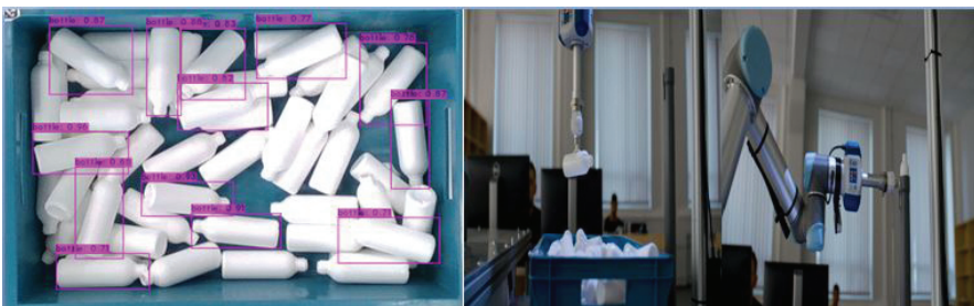
Figure 3.2.4 Object detection and pick and place operation.
