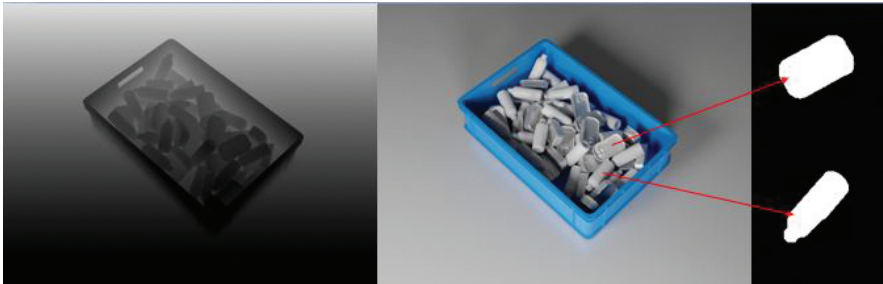
Figure 3.2.6 Scene including the plastic bottle- and the reconstructed metal can 3D models (middle) together with the and corresponding depth image (left) and segmentation masks (right).
