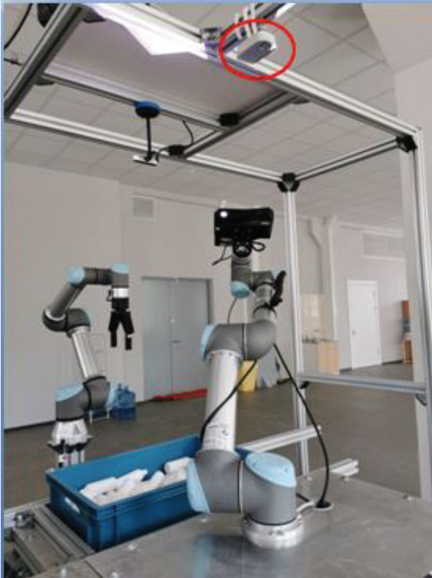
Figure 3.2.5 Setup for object 3D reconstruction.
