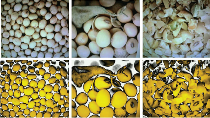
Figure 4.4.8 Image detection segmentation and processing for samples of cleaned soybeans (left), soybeans with impurities (middle) and crushed fractions (right).
