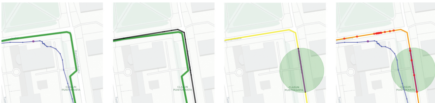
Figure 5.2.7 Refinement of GPS bus traces: (a) Raw GPS [blue] and planned bus route [green] (b) Snapped bus route to OSM road network [black] (c) Partitioned route according to bus stop vicinity [yellow/purple] (d) Map-matching GPS trace [red].
