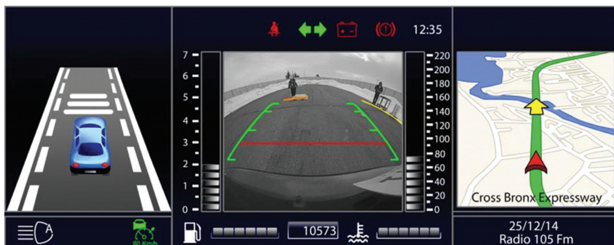
Figure 10.5 Holistic HMI layout with the lane change assist in the central area.
