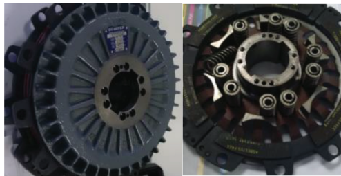
Figure 7.39 GOIZPER pneumatic Clutch Brake outside and inside.
