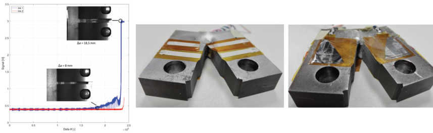
Figure 7.60 Ink signal during the second phase of fatigue test and ink pictures corresponding to the two points indicated in the graph. Pictures of both sides of the test specimen, at the end of the fatigue test.
