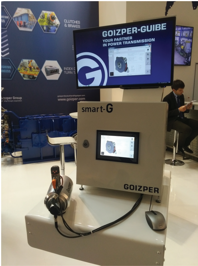
Figure 7.44 Local data logger for data capturing and processing.
