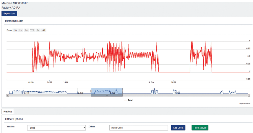
Figure 7.88 Checking the “Bend” variable on a GreenBender machine.
