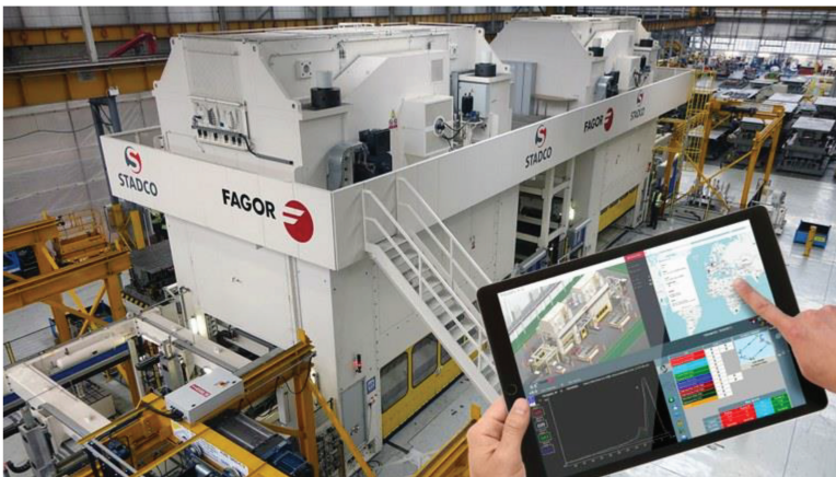
Figure 7.37 Predictive maintenance HMI platform.
