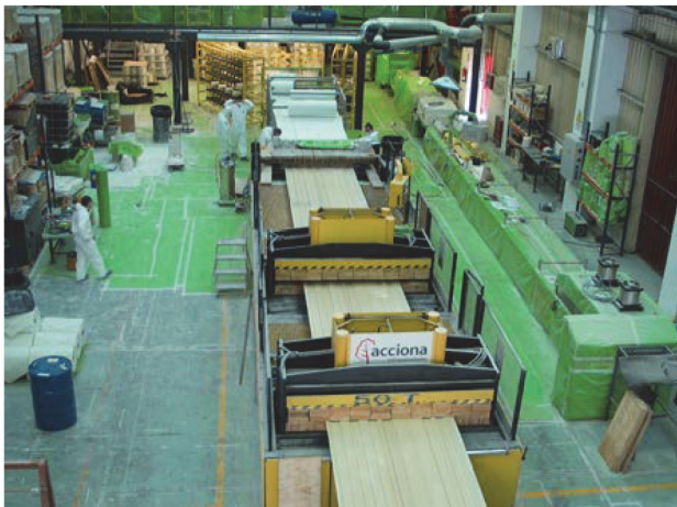
Figure 7.14 Pultrusion machine at ACCIONA workshop.
