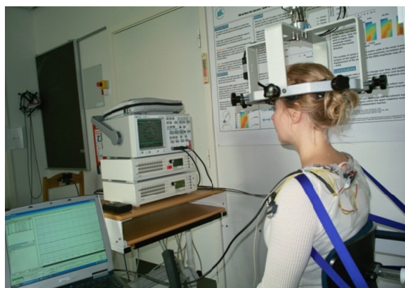
Fig. 28. The subject is sitting with the head fixed in the force device in front of the oscilloscope
