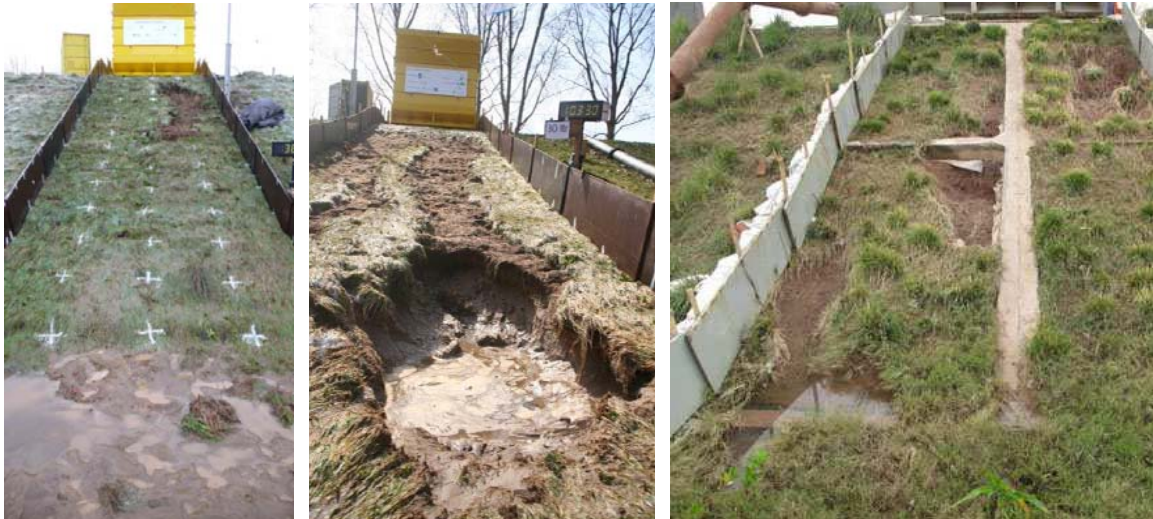
Figure 32. Failures of landward slopes. (left) (Steendam et al., 2011), (middle) (Van der Meer, 2010), (right) (Tung et al., 2012).
