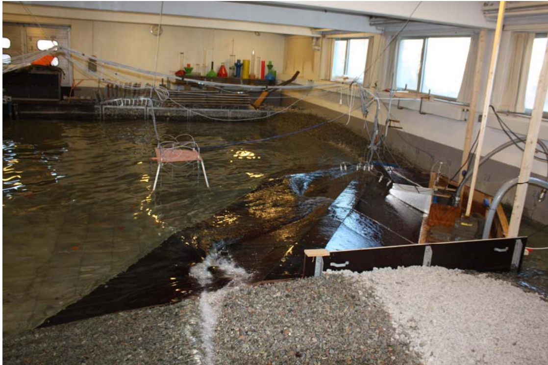
Figure 25. Illustration of Dike Model Setup with and orientation of 37.5° relative to the wave paddles. (Paper 5)
