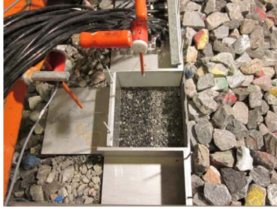
Figure 16. Picture of moveable section in the test setup (the effect of horizontal loading from armor units on the crown wall is not included in the study). (Paper 9)
