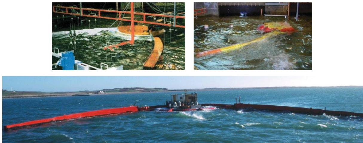
Figure 4. Development stages of Wave Dragon within the Danish Wave Energy Programme. From left to right and from top to bottom, phase 1 (proof of concept), phase 2 (design optimisation) and phase 3 (first prototype sea trials at Nissum Bredning, Denmark) (Wave Dragon, 2013).
