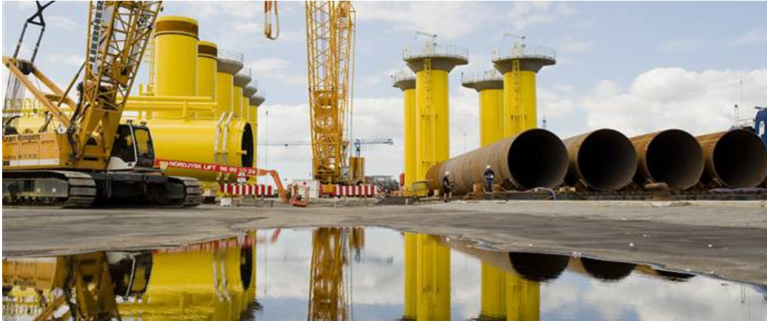
Figure 1.7 Monopile and transition pieces (from www.abjv.com )
