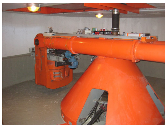
Figure 3.3 Centrifuge at DTU - swing platform with test setup is to the left.
