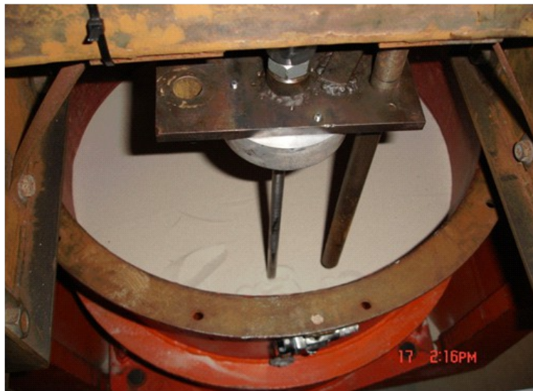
Figure 3.16 Close up of the penetrometer frame with MCP mounted.
