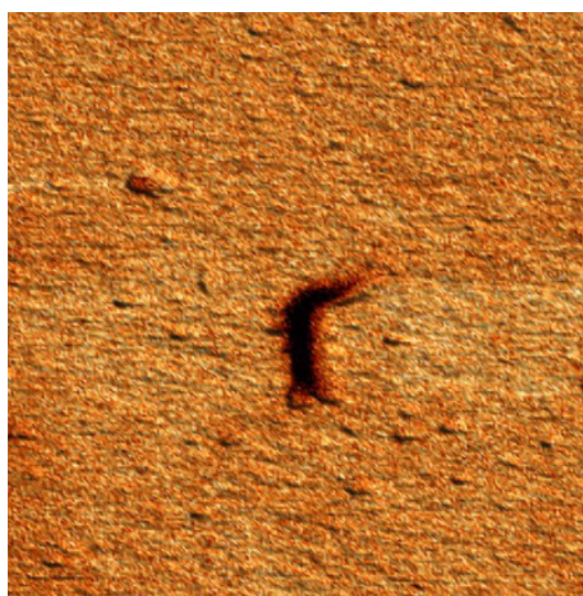
Phase-shift signal produced by KA 6 -coated DNA with the tip bias voltage of -8\text{ V} and lift distance of 50\text{ nm} .
