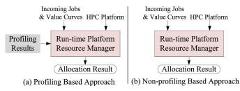
Figure 7.3 Profiling and non-profiling based approaches.
