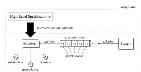
**Figure 3.1** Runtime monitor synthesis and operational set-up.
