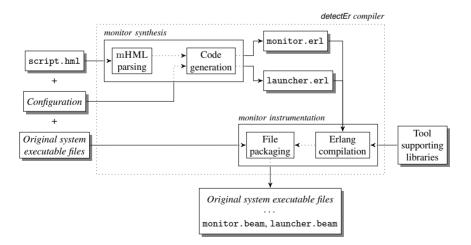
Figure 3.7 The monitor synthesis process and instrumentation pipeline.
