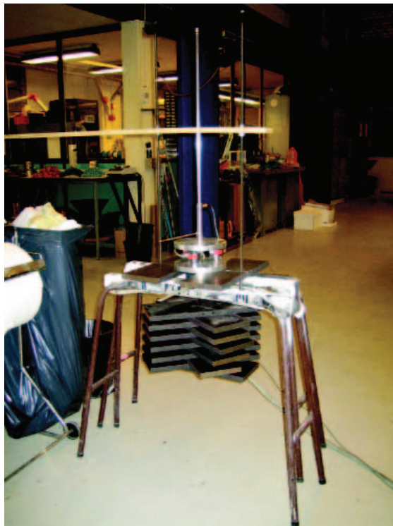
FIGURE 19. SETUP FOR THE CALIBRATION OF THE TIP RESISTANCE OF THE CPT-CONE.
