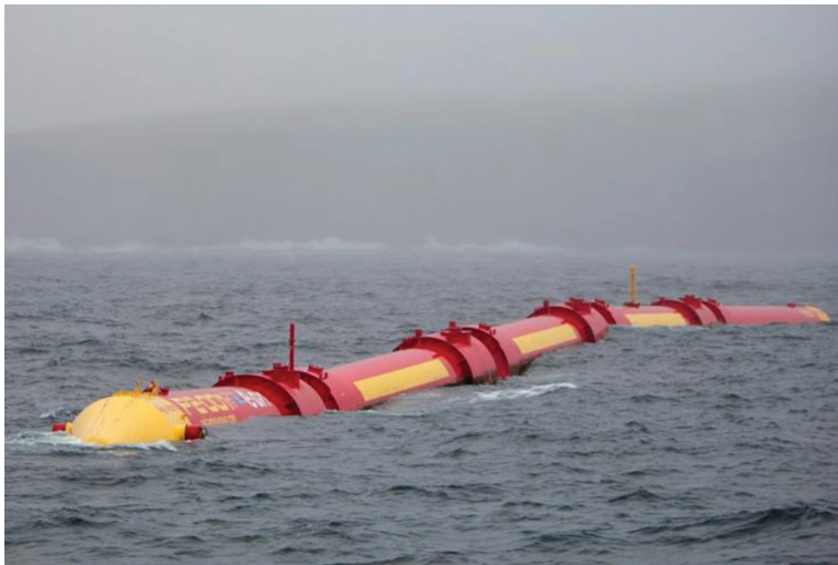
Figure 12.1 Pelamis wave converter Orkney, U.K.
