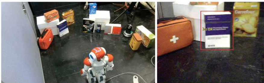
Figure 4.14 Images from a video sequence showing the robot searching for the book (left-side picture) and robot’s camera view and visualization of color interpretation of the searched object (right-side picture).
