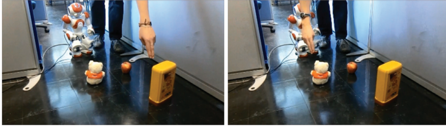
Figure 4.13 Tutor pointing a yellow chocolate box which has been seen, interpreted and learned (by the robot) in terms of colors then asking the robot to describe the chosen object (left-side picture). Tutor pointing an unseen white teddy-bear asking the robot to describe the chosen object (right-side picture).
