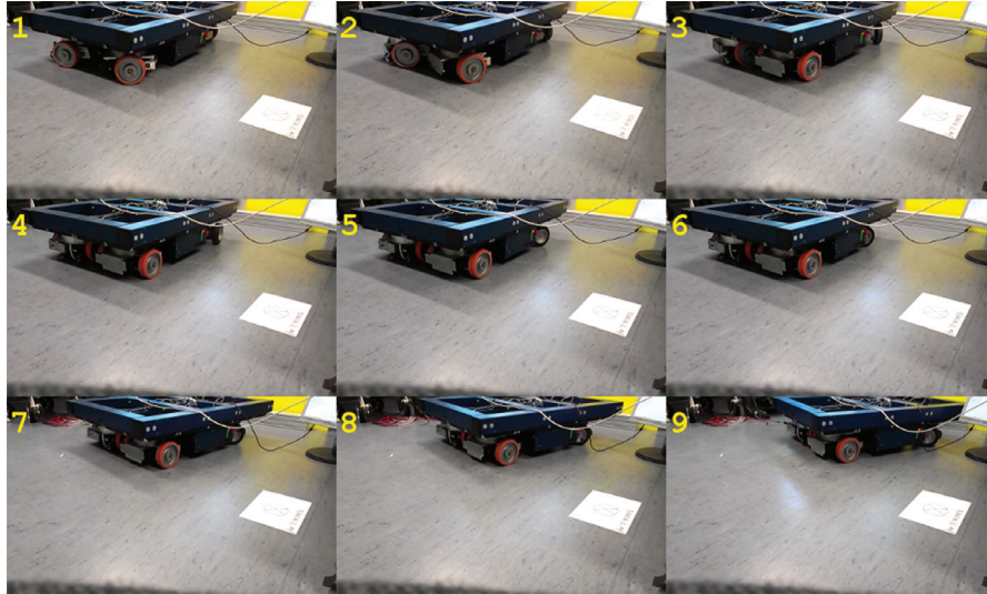
Figure 6.15 The Experiment of modules turning as in the Car Kinematics Scheme (1–6 screenshots) and movement around a White Beacon (7–9).
