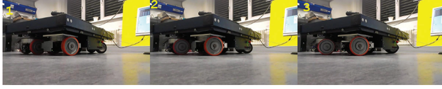
Figure 6.13 Execution of a Learned Control System to turn modules to the center, which is placed on the rear right relative to the platform.
