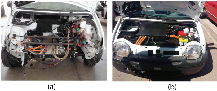
Figure 26 (a) Vehicle front partly disassembled, with battery pack mounting frame and (b) front battery pack integrated.
