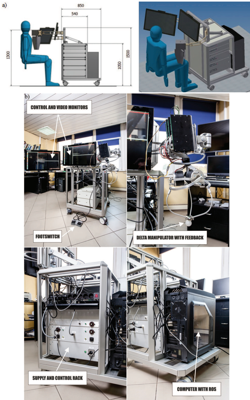
Figure 12.2 STIFF-FLOP console – (a) sketches of design concept and (b) modular prototype with components' description.
