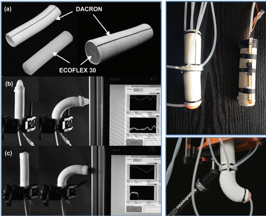
Figure 16.9 The FCSD flexible manipulator inspired by STIFF-FLOP; the construction and the first test of manipulator with pressure and force sensors.
