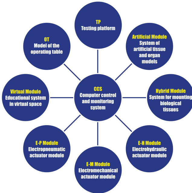
Figure 17.1 STIFF-FLOP robot testing system diagram.
