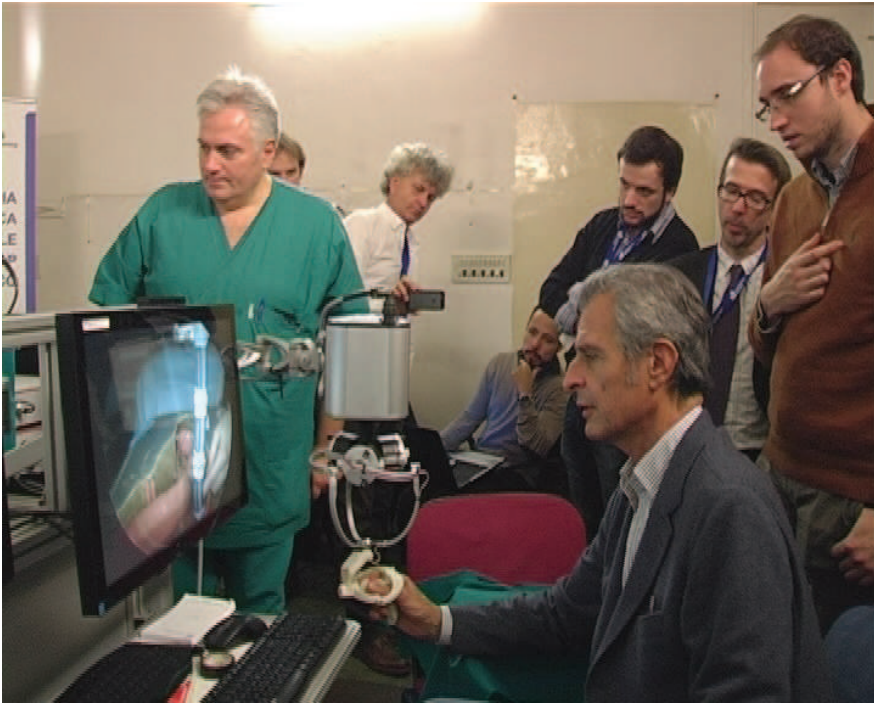
Figure 19.2 Six degrees of freedom (DoF) haptic input device, based on a Delta robot design.
