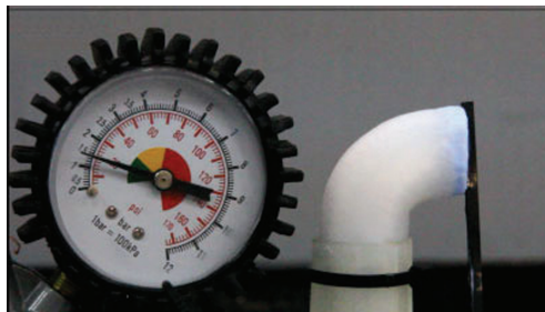
Figure 3.10 Test configuration for measuring module bending by applying pressure into module chambers.
