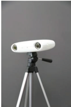
Figure 8.2 Stereo camera Axios Cambar B2, Axios 3D, Oldenburg, Germany.
