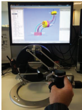
Figure 9.1 Example of a haptic device used to receive the motion request for the robotic tool (Omega 7 from Force Dimension 1 ). For description refer to Chapter 16.
