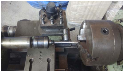
Figure 3. Burnishing tool attached to lathe tool post.
