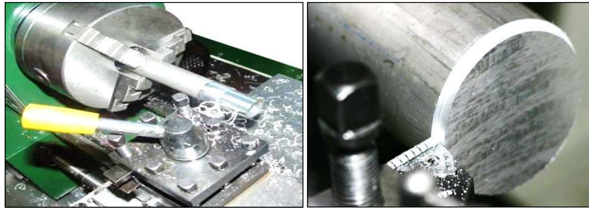
Figure No.2.2 Specimen preparation with turning operations
