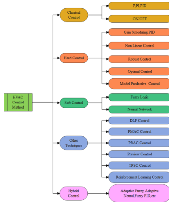
Figure 1 HVAC Control System
