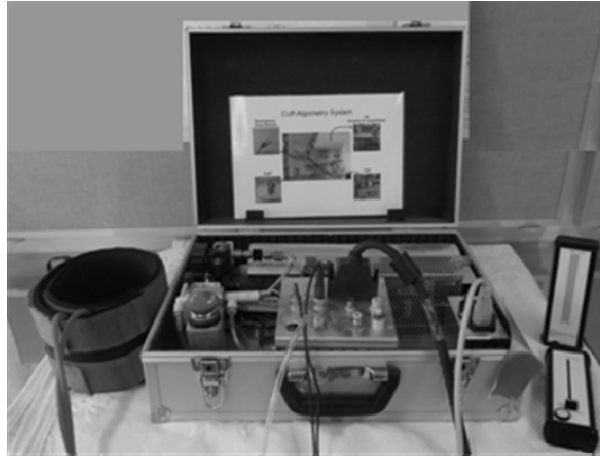
Figure 6. The computer-controlled cuff algometry. Electronic visual analogue scale is shown on the right side.
