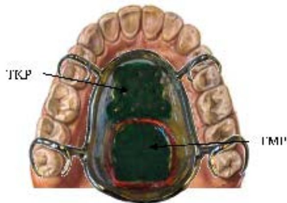
Figure A.1. Palatal interface with inductive sensor boards; The Tongue mousepad (TMP) area contains 8 sensors and the tongue keypad area (TKP) contains 10 round sensors. The TMP is fenced by a charging coil.
