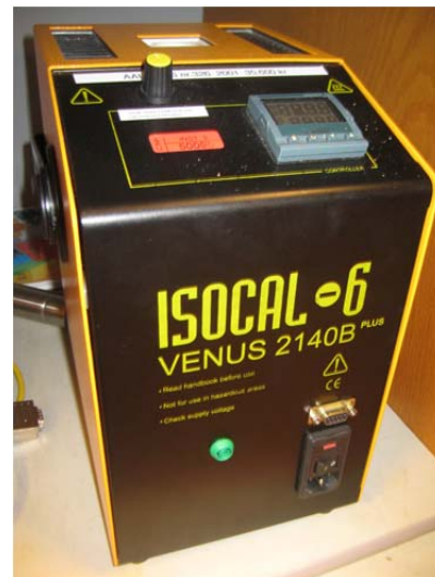
Figure A.1 a) Precision thermometer used for the calibration of the thermocouples, b) Thermal calibration bath, ISOCAL 6
