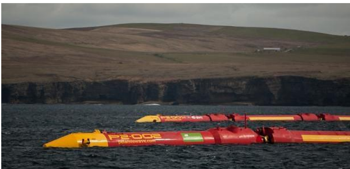
Figure 10: Illustration of Phase 5, array of two Pelamis P2 WECs undergoing trials at EMEC [53].
