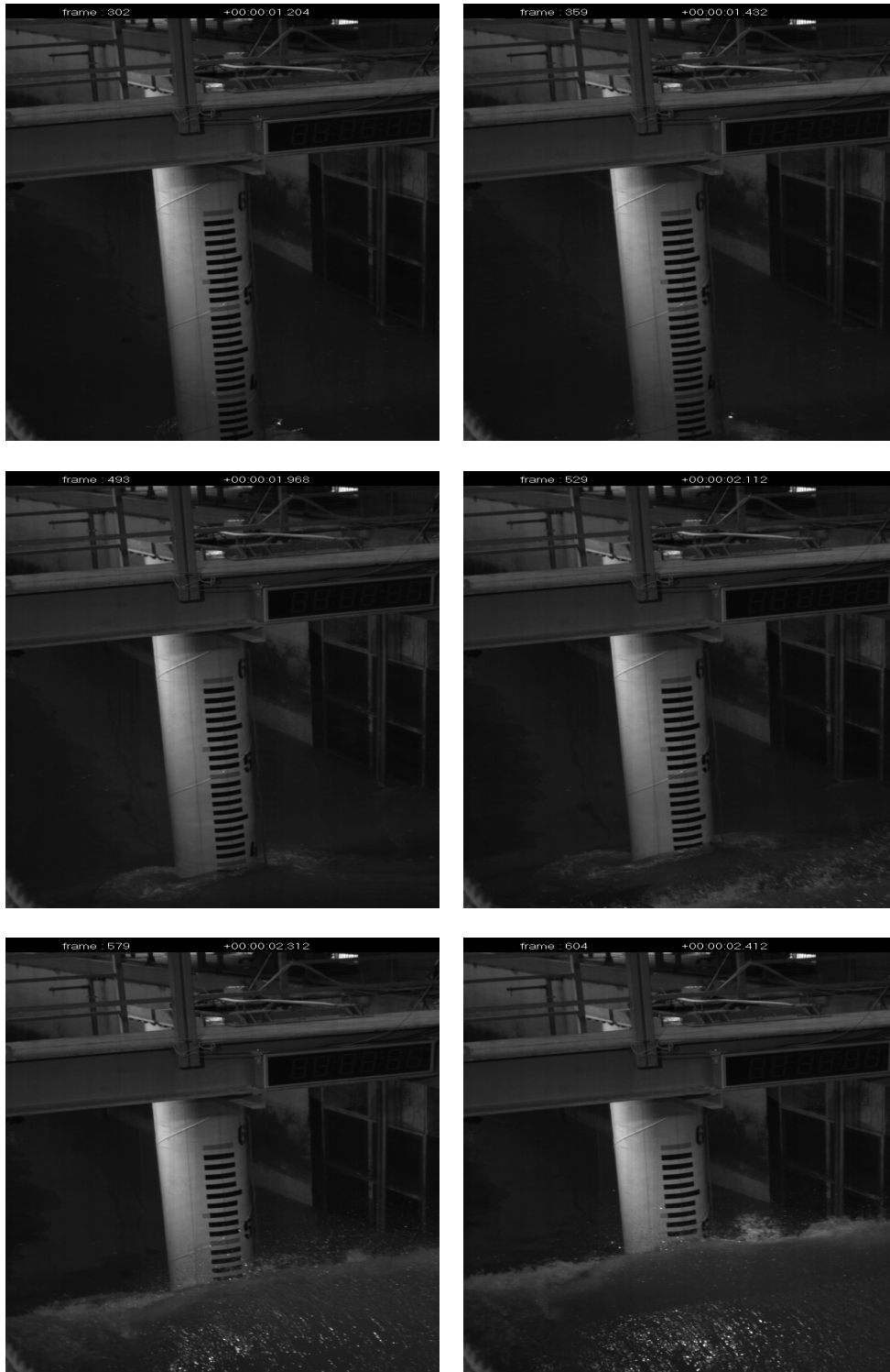
Figure C.2: Snapshot of the breaking waves impacting on the cylinder. Wave cond August, 2012 1.03, T = 4.6
