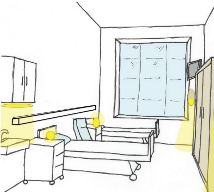
Fig 5.9 Location of luminaires in 'High Lighting Scenario'
