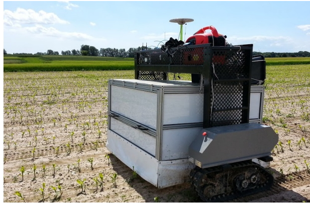
Figure 1.5: Here is an example of a sophisticated computer vision setup. This field robot detects and recognizes plants from weeds to reduce the use of pesticides. Apart from multispectral camera technology, the robot is equipped with Real Time Kinematic-GPS for navigation. Photo by Morten Stigaard Laursen.
