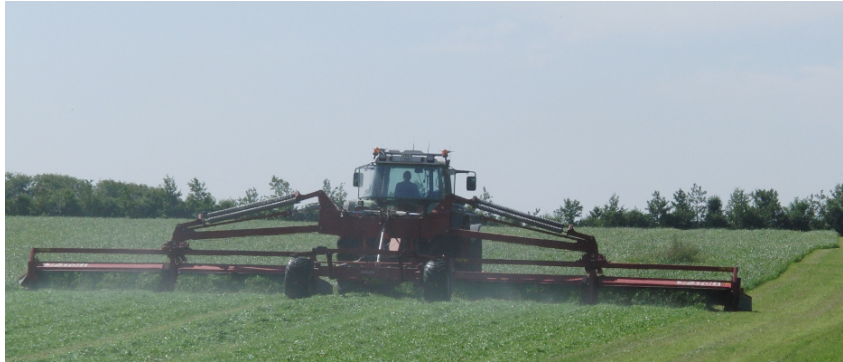
Figure 1.2: An example of mowing operations. The machine in the picture has a typical working width of 14.6 meters and working speeds from 18 km/h to 22 km/h. Photo by Ole Green.
