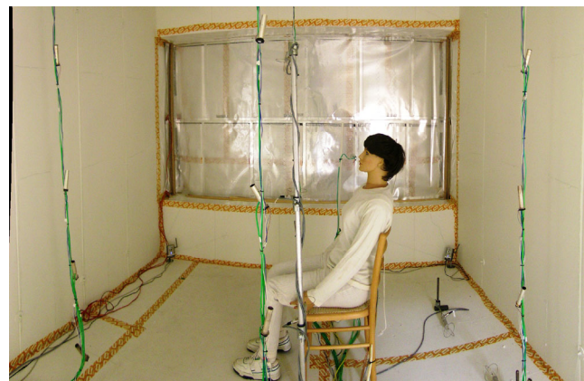
Fig. 4 Panoramic view of the set-up with the electric carpet (steady-state)
