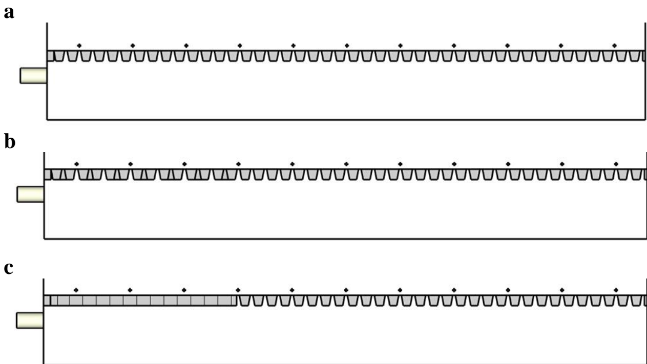
Fig. 2.3 - The three types of floor system: (a) fully slatted floor; (b) 1/3 drain floor + 2/3 slatted floor; (c) 1/3 solid floor + 2/3 slatted floor.
