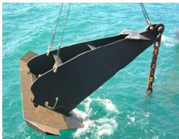
Figure 3: Drag Anchor with studded chain. Source: http://www.vryhof.com .
