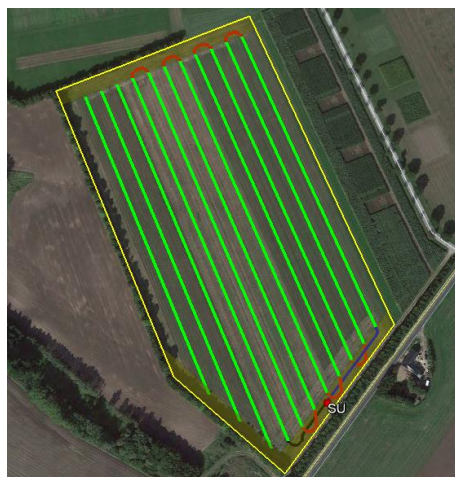
Fig. 1 - Geometrical representation of a field with outer field border (yellow), field tracks (green) in the field body, turnings (red) in the headland areas and refilling path (black) / resuming path (blue) to/from a service unit (SU).
