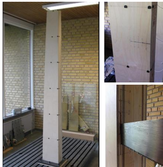
Figure 46. The blade structure. Right top: damage in blade A, Right bottom: damage in blade B
