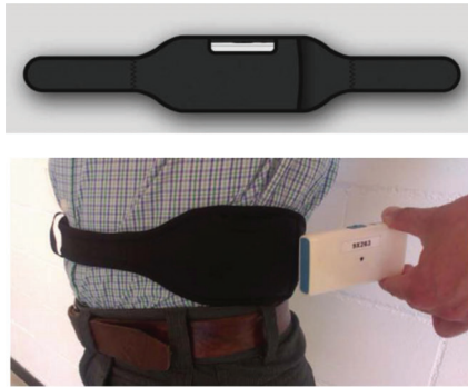
Figure 5.8 Special belt and REMPARK final sensor.
