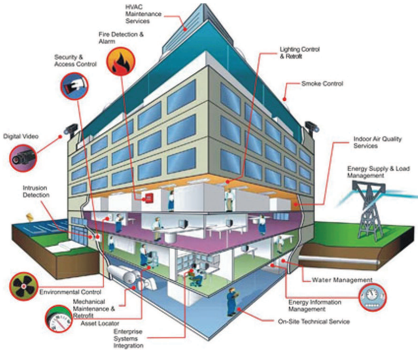
Figure 3.17 Smart building implementation [22].
