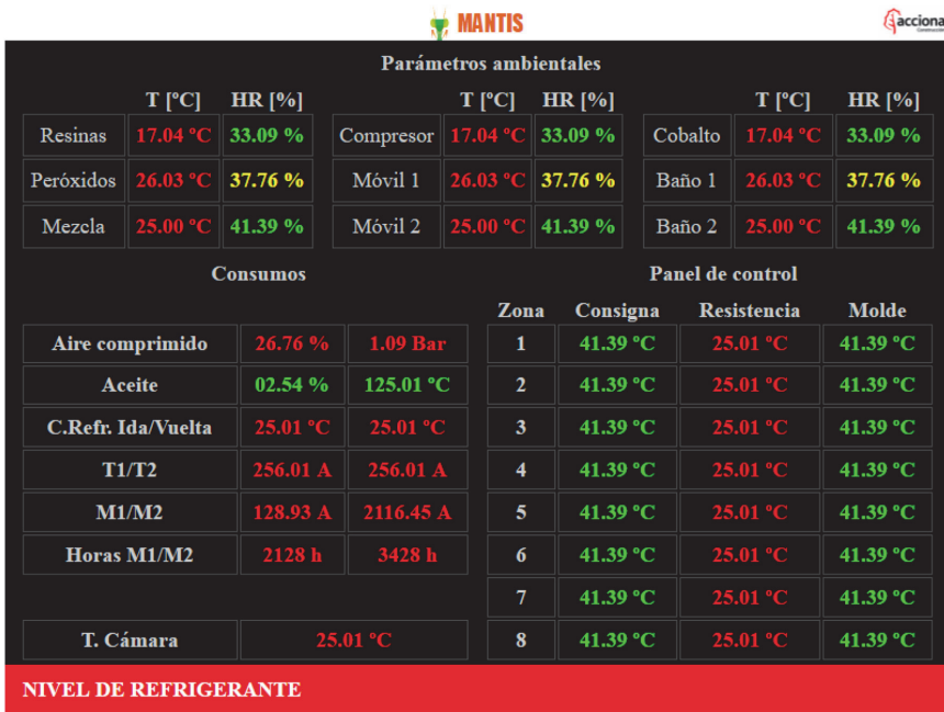
Figure 7.16 Local HMI. PC, Tablets, mobile devices.
