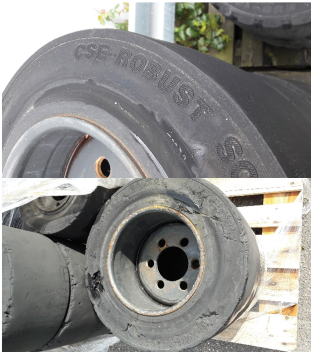
Figure 7.97 Tire changed due to wear and damage.
