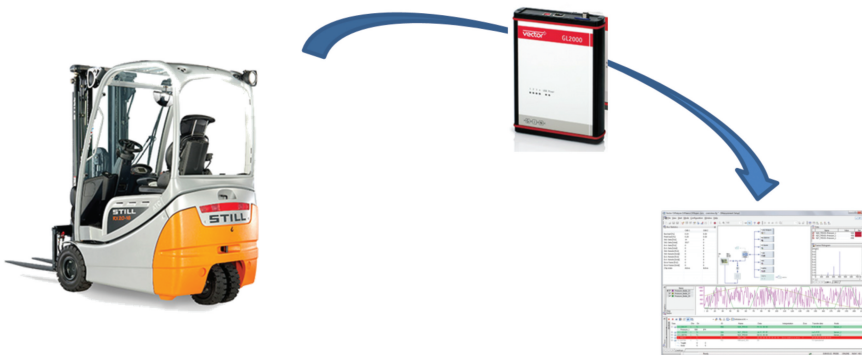
Figure 7.95 Data Logging on the internal CAN bus.
