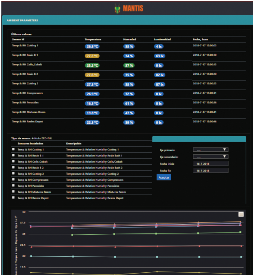
Figure 7.18 Remote HMI. Temperature, Humidity & Light (THL) menu.
