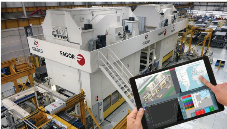
Figure 7.37 Predictive maintenance HMI platform.
