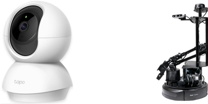
Figure 2.3 Applications: Our agentic system enables active sensing solutions for edge robotics and surveillance IoT cameras. On the left, the Tapo IoT camera [27] is used for surveillance applications. On the right, the Locobot robot WX250 [28] for information gathering and scene discovery.
