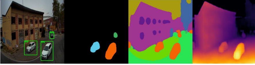
Figure 11.1 Sample outputs for the Multi-task perception pipeline deployed in a smart-city scenario. Right to Left: object detection, instance segmentation, semantic segmentation, and monocular depth estimation.
