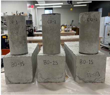
Fig. 2 Cylinder & Beam Specimens
