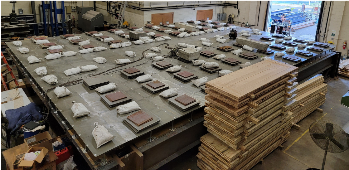
Fig. 4 Configuration with service load (SL) applied as distributed mass simulating a 12 psf area load
