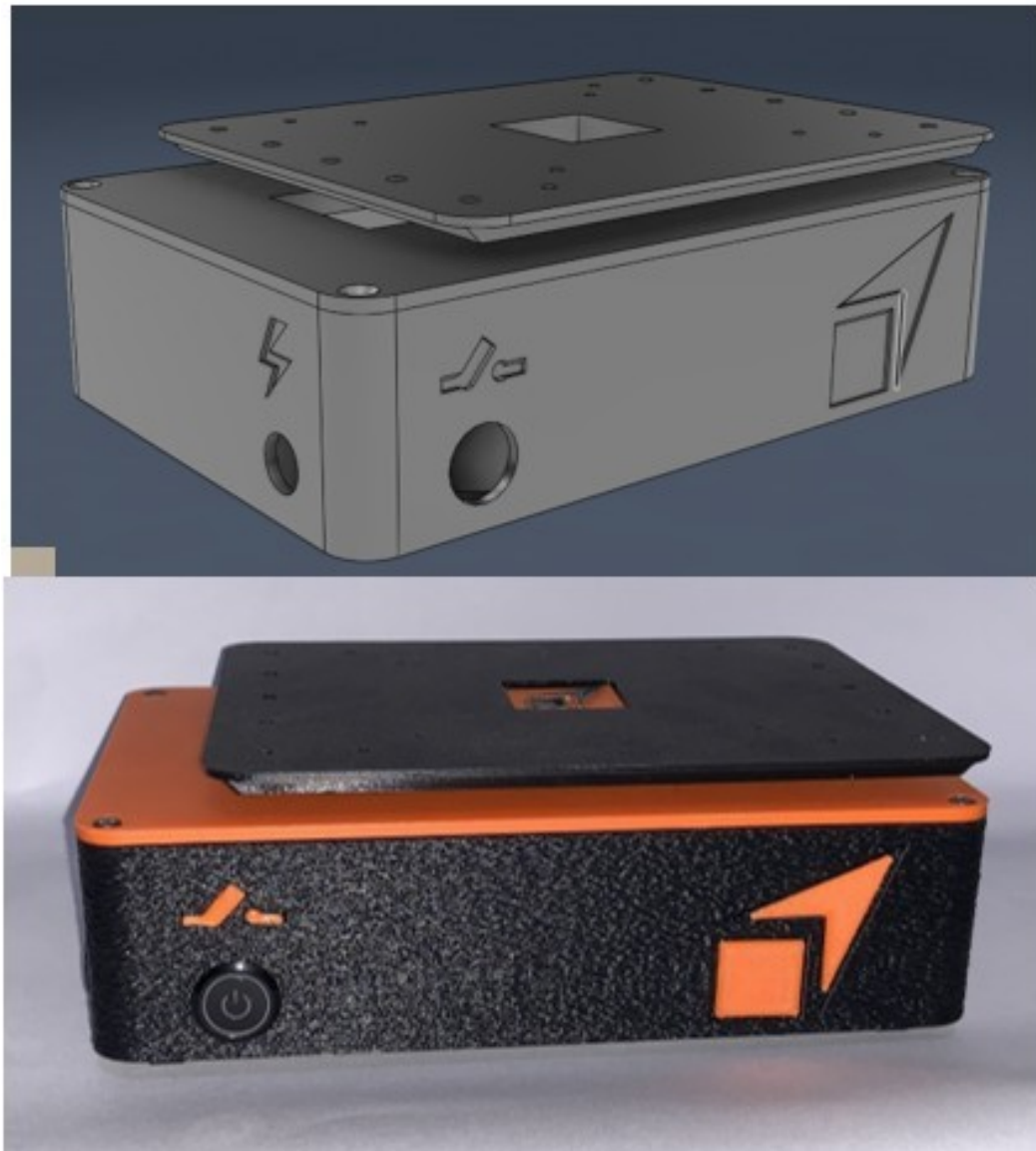
Fig. 1 Design and execution of the P-Shaker in PLA
